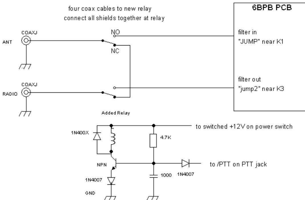
With this arrangement, when the power is off, or when PTT is asserted, the relay is de-energized and bypasses the filter. Because of the short connections, the swr thru the filter is now less than 1.3 to 1 from 160-10M when it is off. When the power is turned on, the relay is energized, and the filter will be “in-line”.
